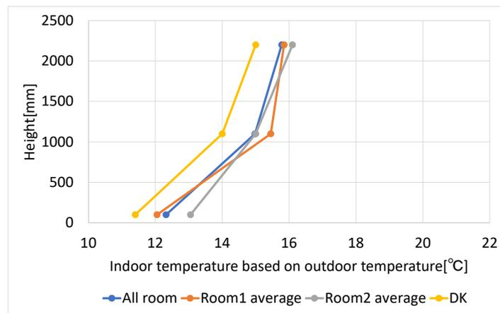
Fig 7. Case1 Vertical temperature distribution (Field measurement)
