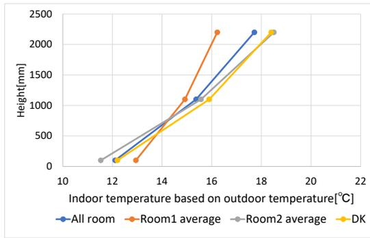
Fig 20. Case4 Vertical temperature distribution (CFD)
