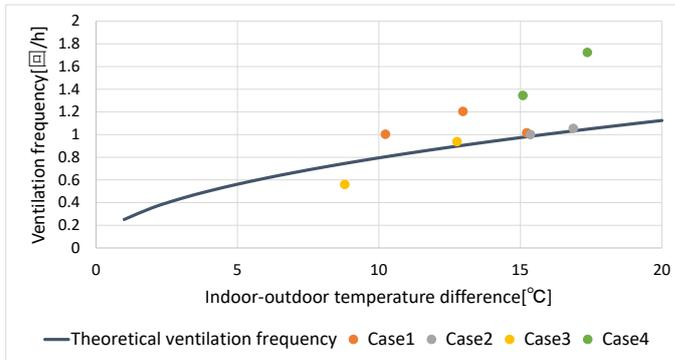
Fig5. Comparison of measured and theoretical ventilation frequency results
