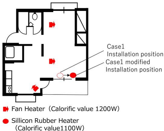
Fig 25. Case1 modified Heating element location
