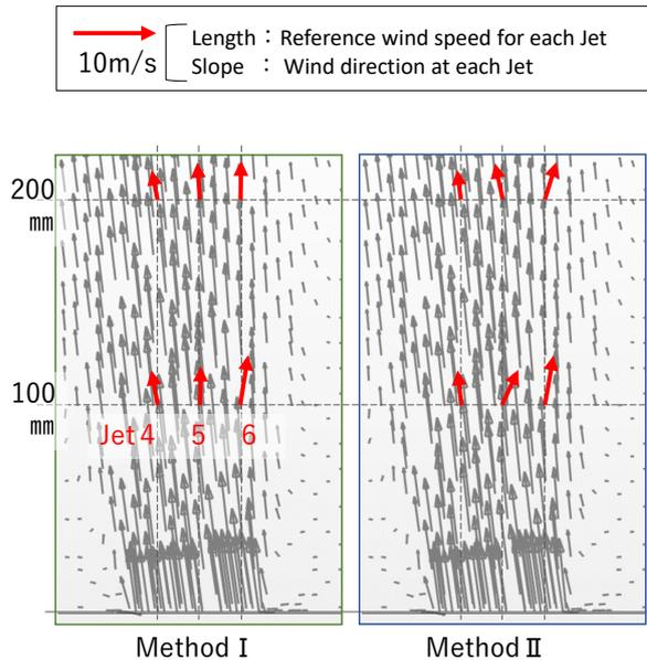
Fig11. Comparison of wind direction (yaw angle)
