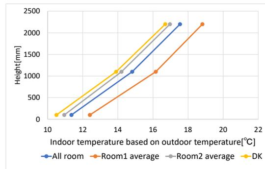
Fig 19. Case2 Vertical temperature distribution (CFD)
