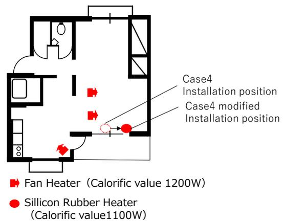
Fig 26. Case4 modified Heating element location
