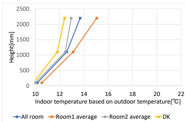
Fig 11. Case3 Vertical temperature distribution (Field measurement)
