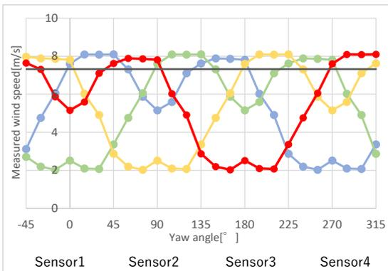
Fig 6. Indicated value of each sensor ( $0^\circ$  pitch angle)
