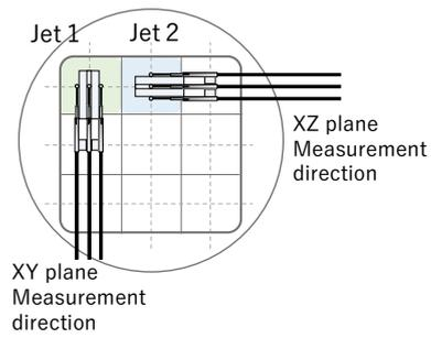
Fig 4. Measuring Method with Quad-Thermistor
