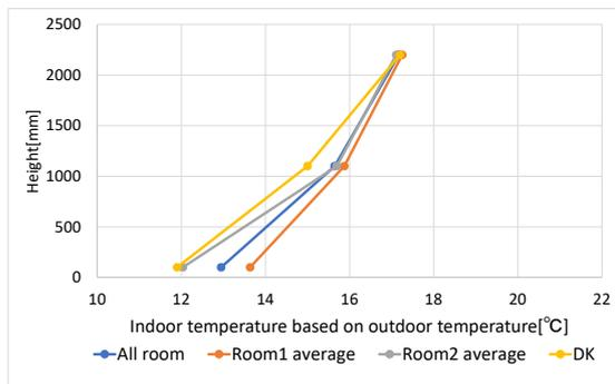
Fig 18. Case1 Vertical temperature distribution (CFD)
