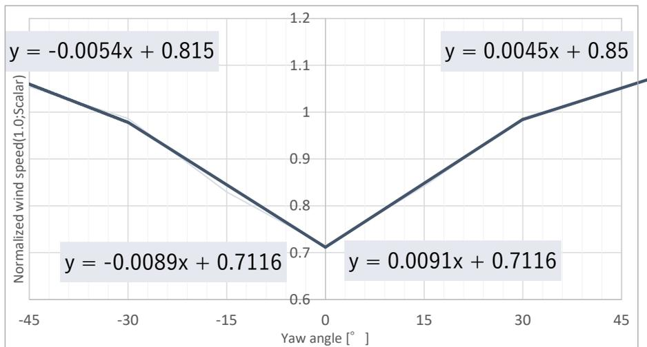
Fig 9. 【Calculation Method II】 Standardized Approximate Line ( $-45^\circ \leq \theta \leq 45^\circ$ )
