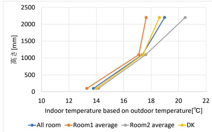
Fig 13. Case4 Vertical temperature distribution (Field measurement)
