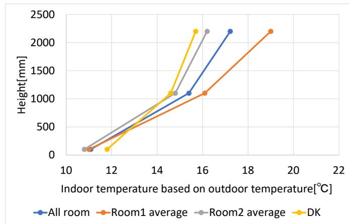
Fig 9. Case2 Vertical temperature distribution (Field measurement)
